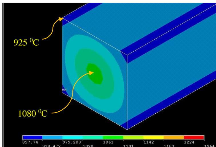
Figure 3 Temperature profile after 50 seconds from CCM cut
