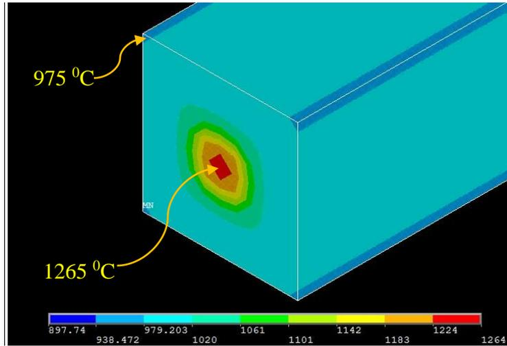
Figure 1 Temperature profile after 5 seconds from CCM cut
