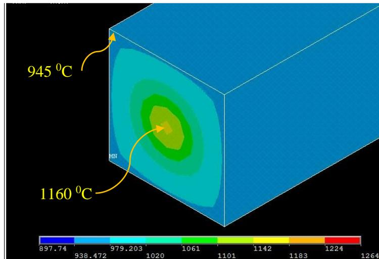
Figure 2 Temperature profile after 20 seconds from CCM cut
